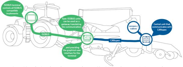
Epec EC44 Agri Control Unit can be used as a gateway between ISOBUS and another communication protocol.
