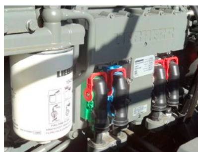
Diesel engine ECU with inbuilt cable clamps. (Image courtesy of TE Connectivity)
