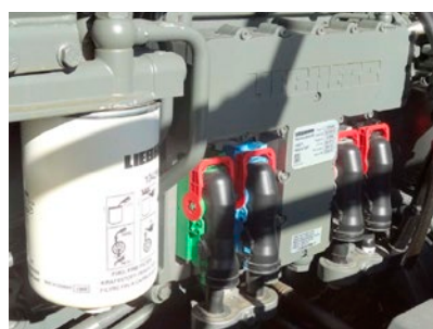
Diesel engine ECU with inbuilt cable clamps. (Image courtesy of TE Connectivity)
